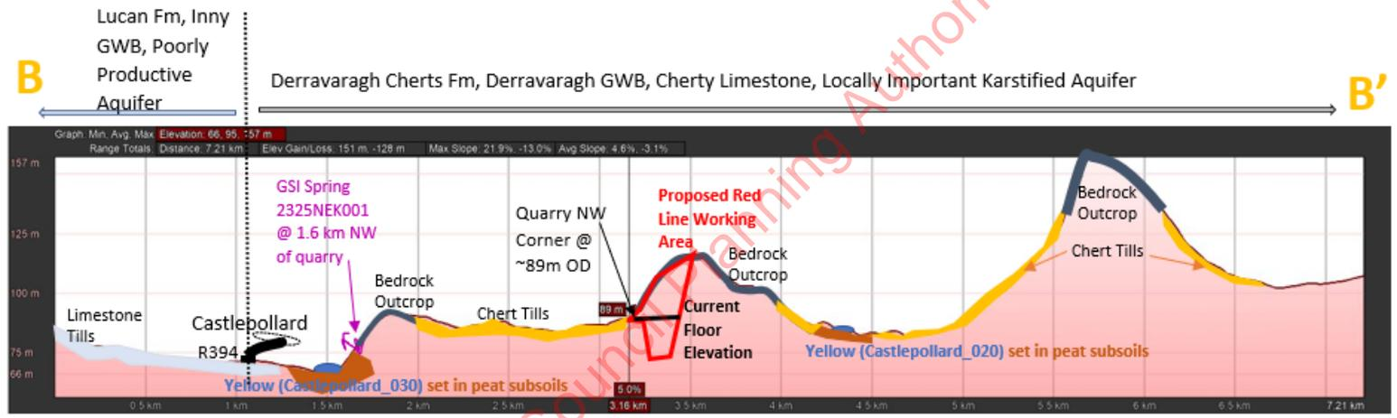
Plate 7.5 (c) Cross Section Northwest to Southeast B-B' (base section source Google Earth Pro, annotated by Hydro-G)
